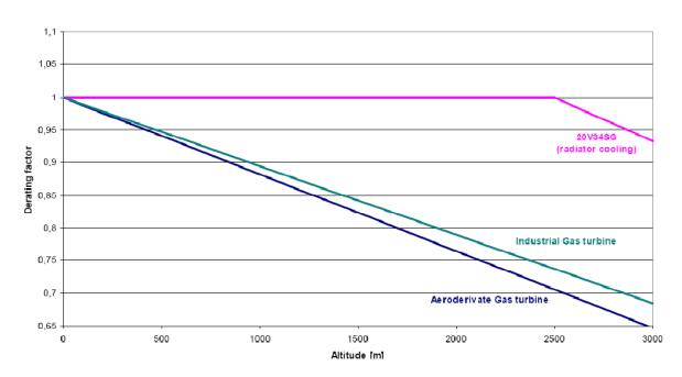
• Figure 4 General altitude de-rating factors for typical gas turbines
