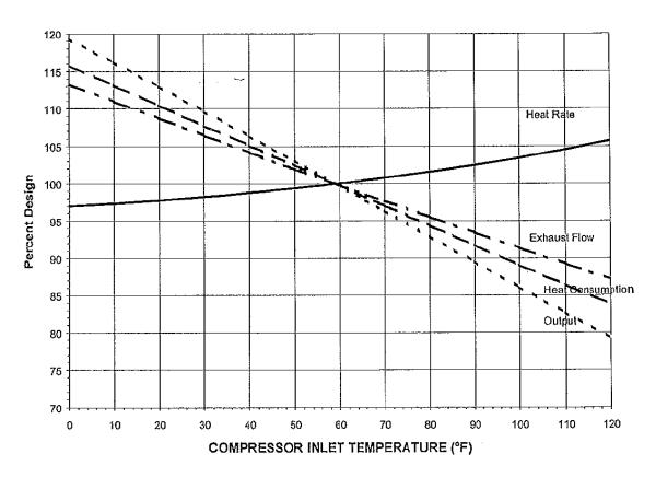
Figure 5 Typical Generator Performance Graph Provided by Manufacturers
