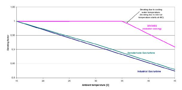
Figure 3 General ambient de-rating factor for typical gas turbines
