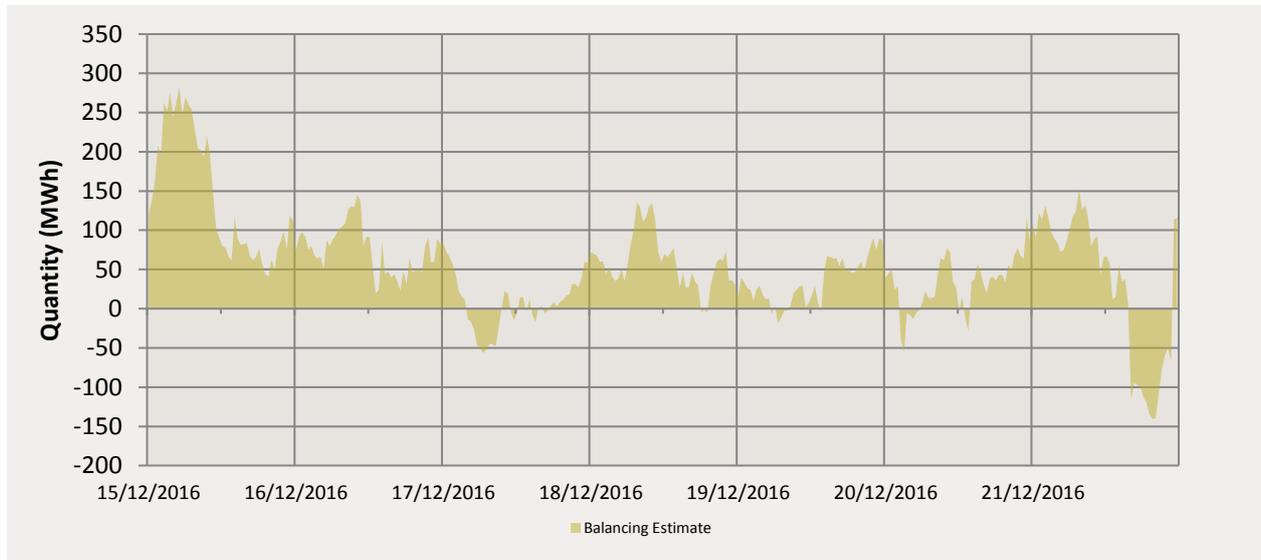
The majority of the balancing activity this week occurred within Balancing Demand. The maximum balancing demand for the week reached 281.778 MWh on the 15/12/2016. The maximum balancing supply for the week reached -140.773 MWh on the 21/12/2016.
