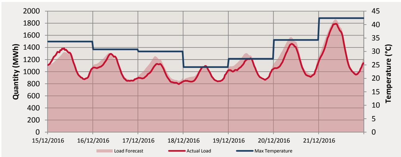
The maximum temperatures for this trading week ranged from 24.2°C to 42.4°C. The actual load peaked at 1791.391 MWh on the 21/12/2016.
