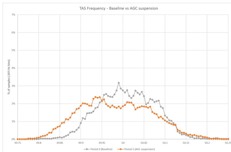
**Figure 3.8 Frequency histograms for baseline and AGC suspended test periods**
