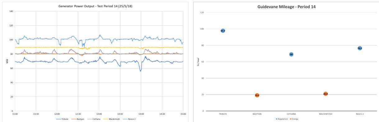
Figure A.32 Monitored generator power output and guide vane mileage - test period 14
