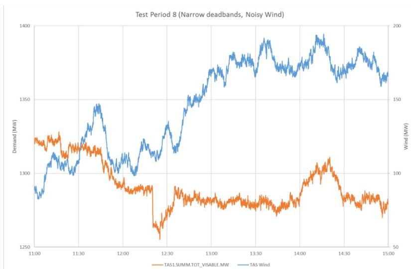
**Figure 3.5 Tasmanian demand and total wind generation during test period 8**
