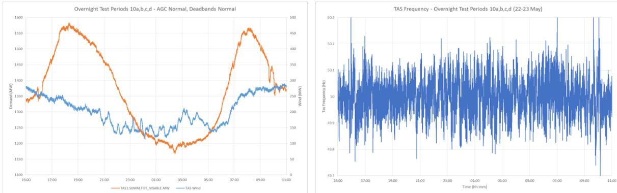
**Figure A.20 Tasmanian demand, total wind generation and frequency - test period 10**
