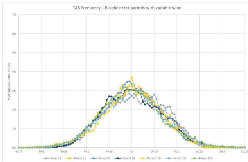
**Figure 3.1 Baseline test frequency distributions with variable wind generation**
