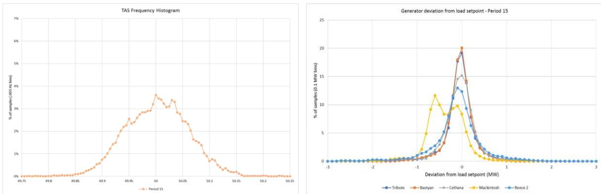
Figure A.34 Tasmanian frequency and deviation from load setpoint histograms - test period 15
