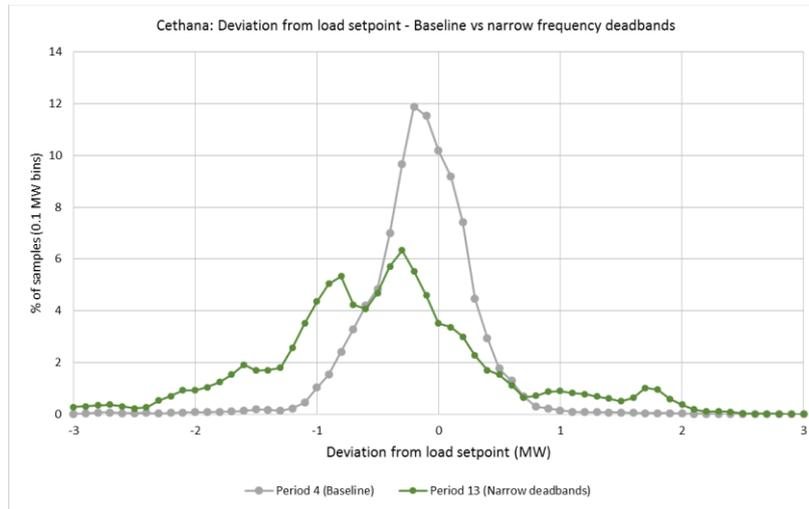
**Figure 3.11 Cethana deviation from load setpoint histogram- baseline vs narrow deadbands**
