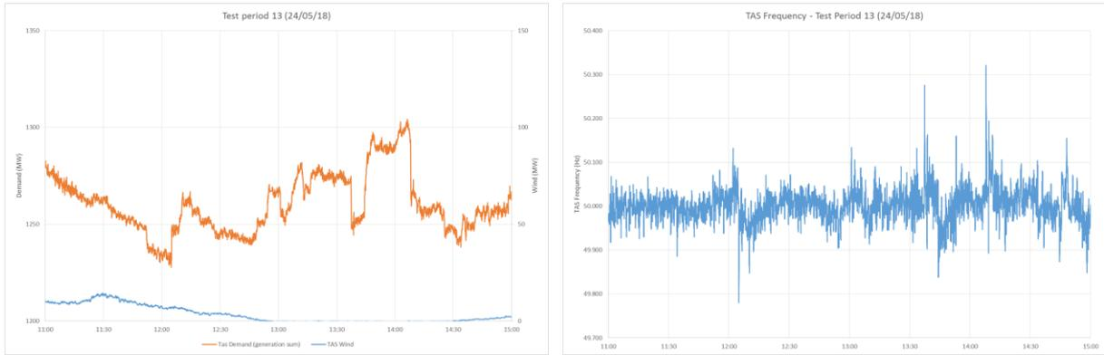
Figure A.27 Tasmanian demand, total wind generation and frequency - test period 13
