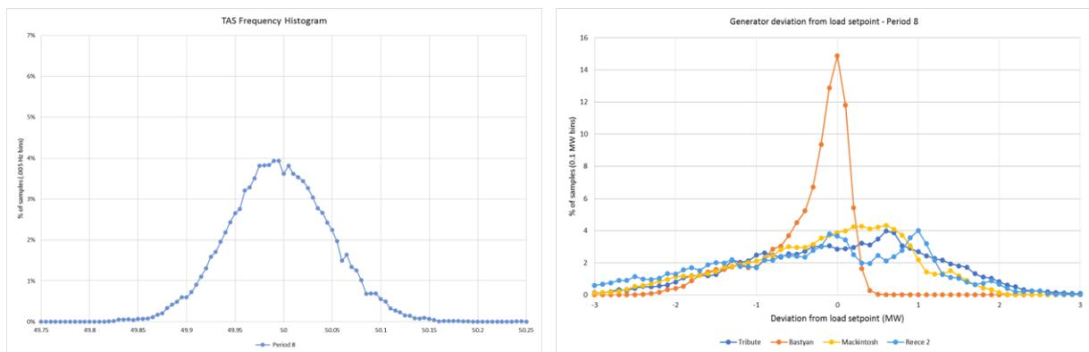
Figure A.15 Tasmanian frequency and deviation from load setpoint histograms - test period 8
