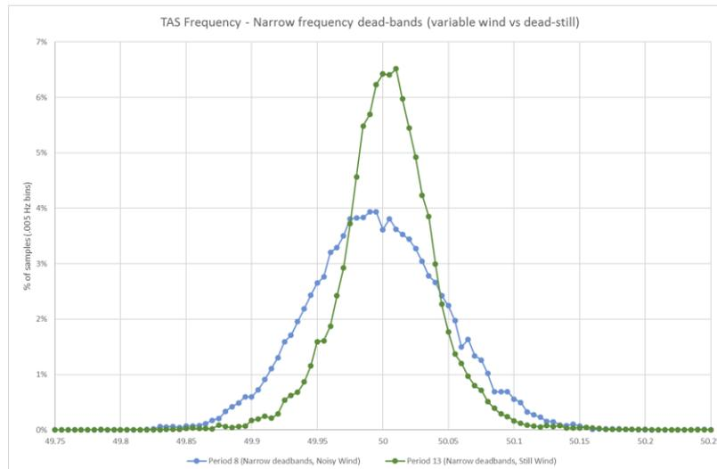
**Figure 3.4 Frequency histograms for narrow deadbands with variable and still wind generation**
