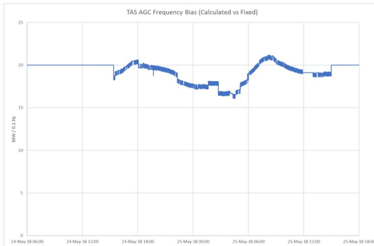
**Figure 3.10 Normal and dynamically calculated AGC bias setting**
