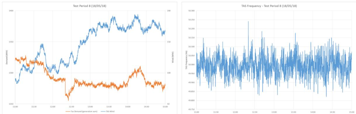
Figure A.14 Tasmanian demand, total wind generation and frequency - test period 8
