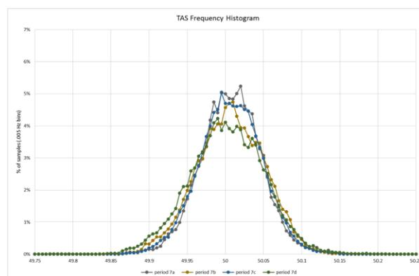
**Figure A.13 Tasmanian frequency histogram - test period 7**
