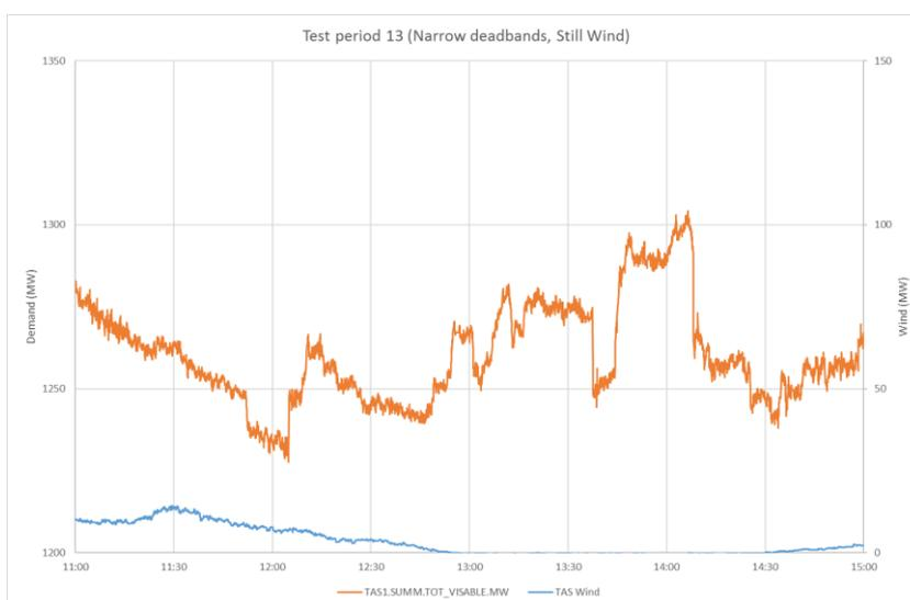
**Figure 3.6 Tasmanian demand and total wind generation during test period 13**
