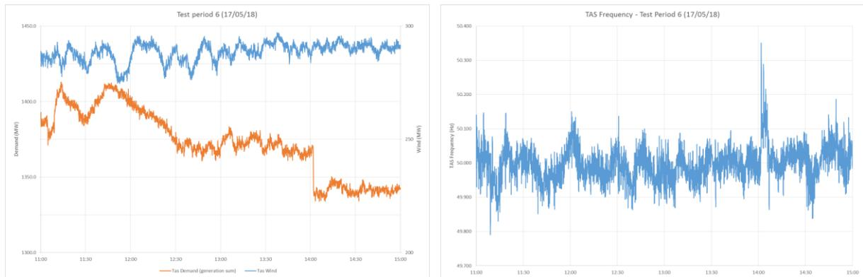
Figure A.9 Tasmanian demand, total wind generation and frequency - test period 6
