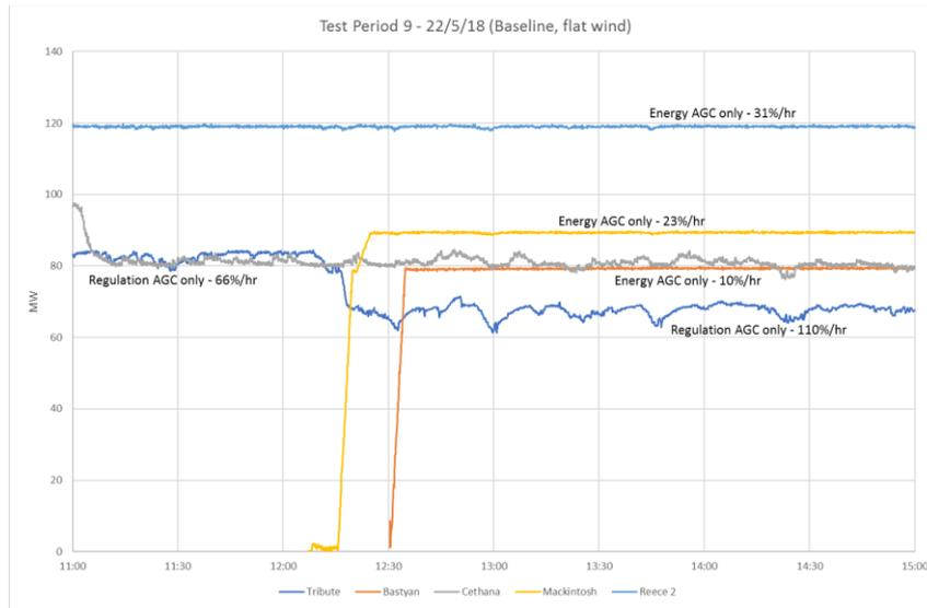
**Figure 3.14 Power output of monitored generators for test period 9**
