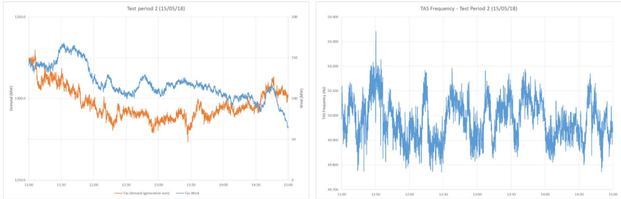
**Figure A.1 Tasmanian demand, total wind generation and frequency - test period 2**
