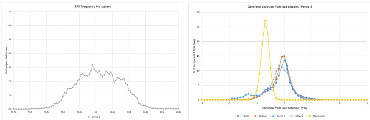
**Figure A.5 Tasmanian frequency and deviation from load setpoint histograms - test period 4**
