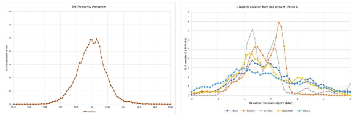
Figure A.10 Tasmanian frequency and deviation from load setpoint histograms - test period 6
