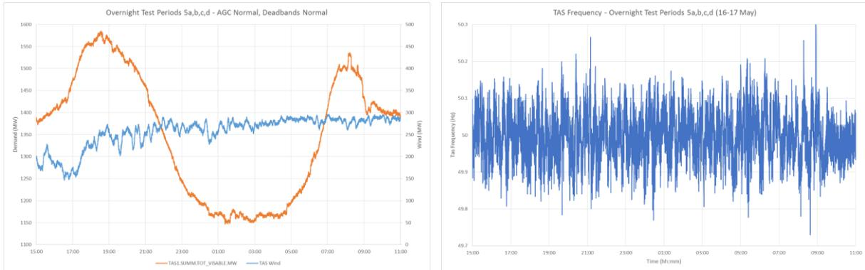
**Figure A.7 Tasmanian demand, total wind generation and frequency - test period 5**
