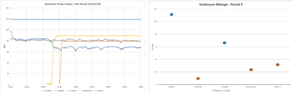
Figure A.19 Monitored generator power output and guide vane mileage - test period 9
