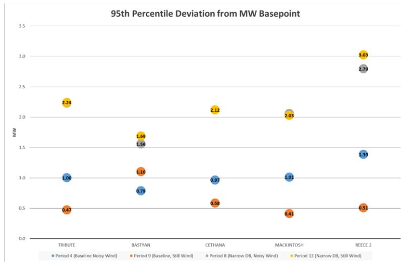
**Figure 3.13 Deviation from load setpoint 95<sup>th</sup> percentiles**
