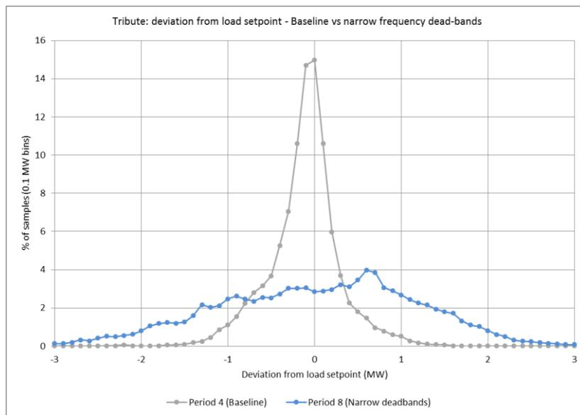
**Figure 3.12 Tribute deviation from load setpoint histogram- baseline vs narrow deadbands**
