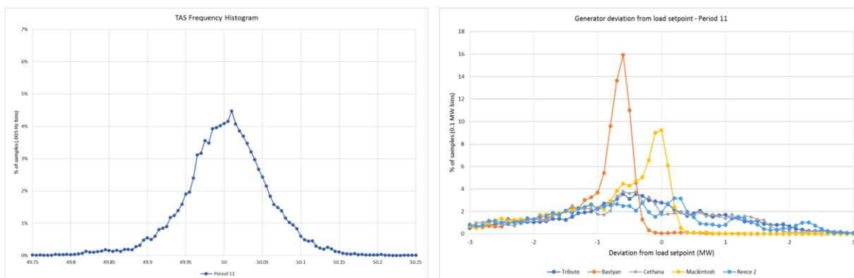
Figure A.23 Tasmanian frequency and deviation from load setpoint histograms - test period 11
