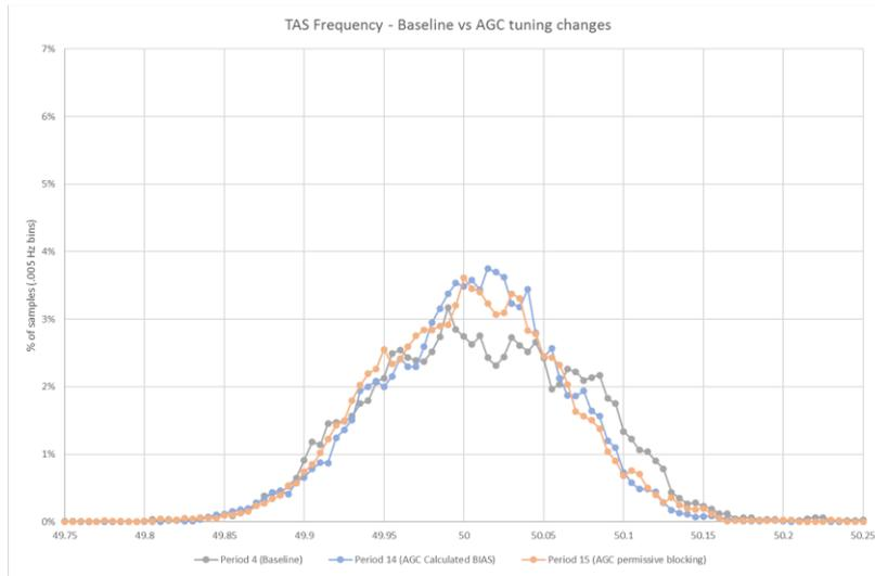
**Figure 3.9 Frequency histogram for AGC settings changes and baseline tests**
