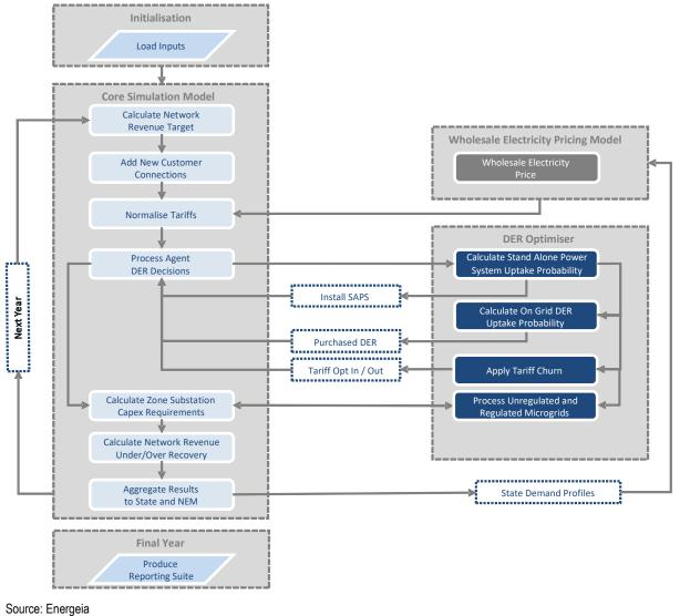
Figure 43 – Overview of DER Simulation Platform
