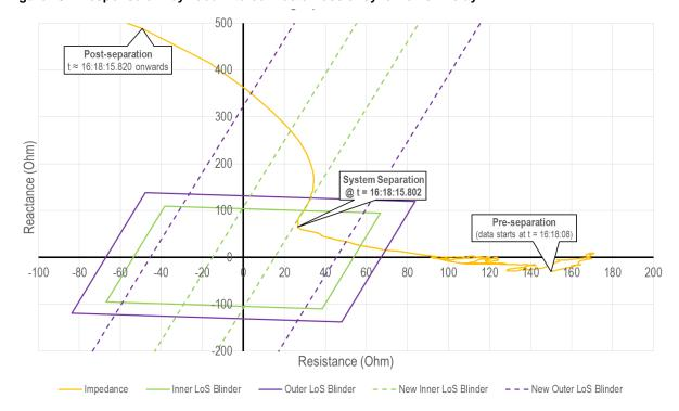
Figure 15 Response of Heywood Interconnector loss of synchronism relay
