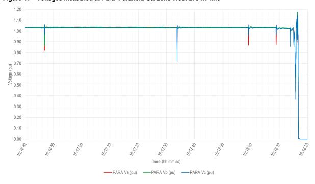
Figure 42 Voltages measured at South East-Tailem Bend No. 1 275 kV line
