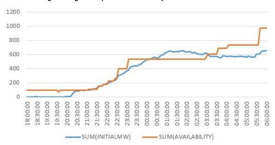
Figure 24 Total unit generating MW output versus availability
