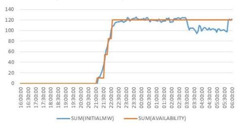
Figure 114 TIPS A4 Generating Unit MW output during restoration
