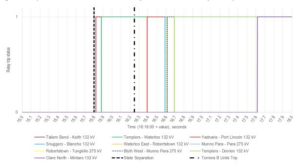
Close inspection of relay data indicates that all these relays operated on three-phase distance protection. However, as discussed in this report, all six voltage disturbances were unbalanced, for which operation of three-phase distance relays should be prevented.
