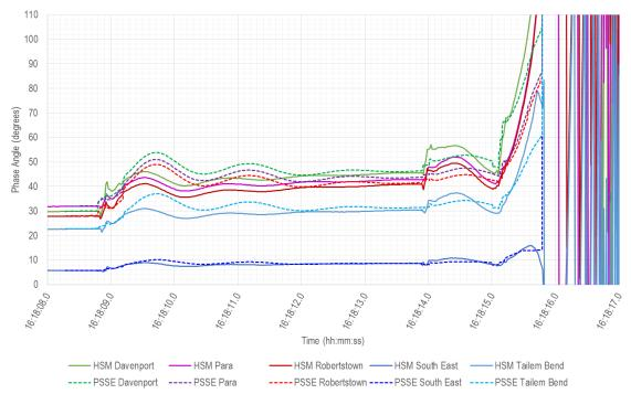
In Figure 137, differences can be observed between the modelled and measured (HSM) values of the Davenport frequency. This stems from the inability of the PSS/E and most other simulation tools to calculate the frequency under extreme operating conditions with abrupt changes in both voltage and frequency. This difference has no material impact on predicting whether loss of synchronism and islanding conditions will occur.
