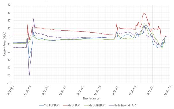
Figure 191 Comparison of reactive power responses at the connection point and that provided by the dynamic reactive support plant
