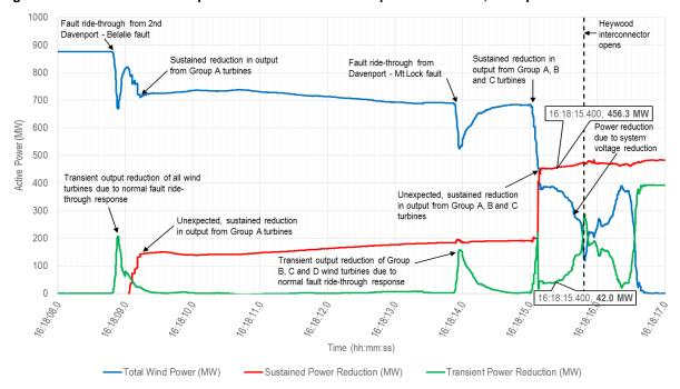
Figure 11 illustrates the power reduction of wind farms, based on the grouping in Table 9. It also highlights the following observations (noting the SA power system had experienced three voltage disturbances just prior to the time shown on Figure 11):
