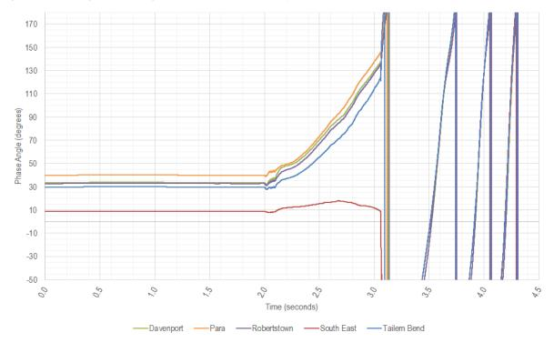
Note that large spikes seen at 3.1 seconds in Figure 158 stem from the inherent inability of simulation tools to track the abrupt changes in voltage phase angles and RoCoF.
