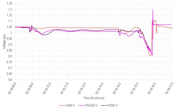
Figure 146 shows a good match between modelling and measured (HSM) values, except for the PSS/E result for peak power flow. This difference has no material impact on predicting whether loss of synchronism and islanding conditions will occur, as this is determined by the impedance trajectory. In Figure 135 and Figure 140, close alignment between the measured and simulated impedance trajectories can be observed.
