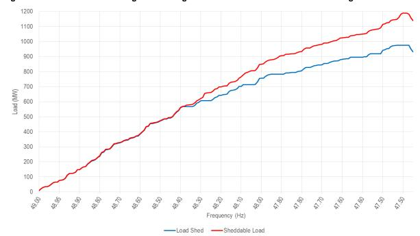
Figure 19 Total load shed during the event against total load available for load shedding
