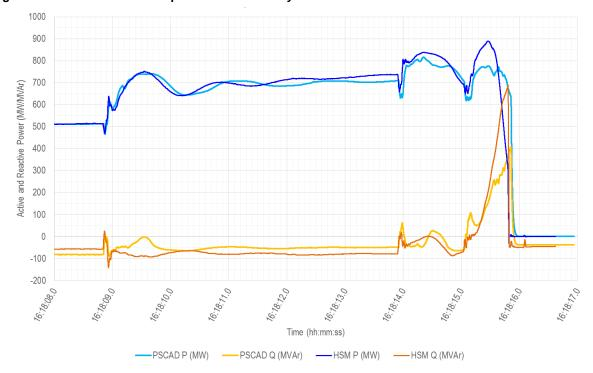
Figure 140 shows a good match between modelling and measured (HSM) values where both the measured and simulated impedance trajectories enter the inner blinder of the Heywood LOS relay, confirming correct and intended operation of this relay.
