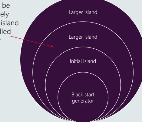
With large quantities of uncoordinated DER, it may become increasingly difficult to anticipate the quantity of load being added to the island. Feed-in management offers a solution, if suitably designed.
