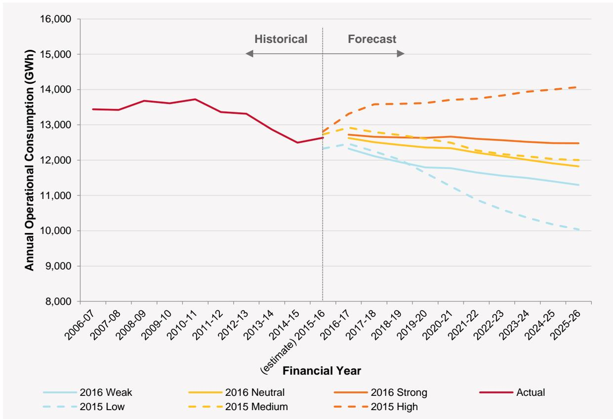
**Figure 2 Annual operational consumption forecast by segment for South Australia (Neutral sensitivity)**
