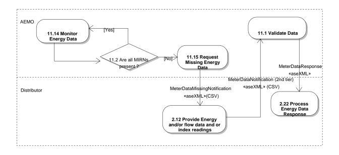
FIGURE 4-25. DELIVERING ENERGY DATA ACTIVITY DIAGRAM
