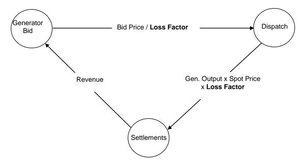
Figure 13: Relationship between bidding, dispatch and settlements
