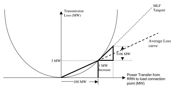
Figure 7 represents the transmission loss versus power flow characteristic for the radial network example shown in Figure 3.
