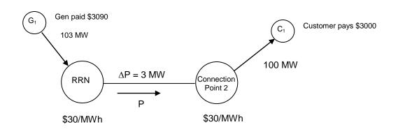
Figure 9: Pool clearance (No loss factor applied)
