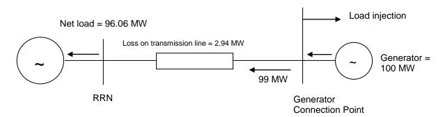
Figure 6: Radial network after 1 MW load injection at generation connection point
