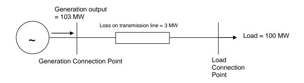
Figure 3: Radial network prior to 1 MW load injection at load connection point
