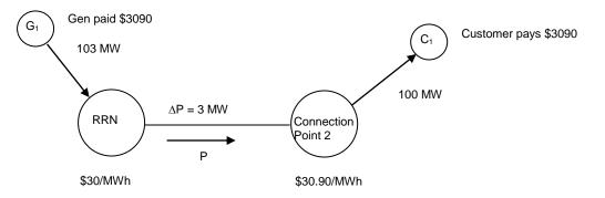
Figure 10: Pool clearance (Average loss factor applied)
