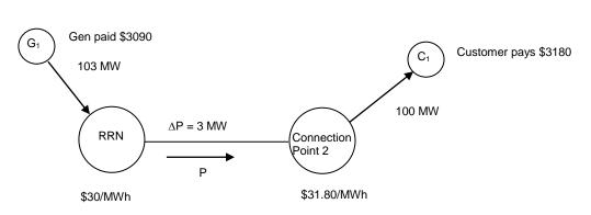
Figure 11: Pool clearance (Marginal loss factor applied)
