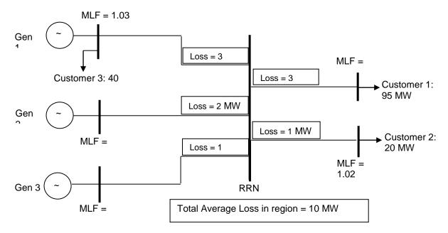
Figure 12: Dispatch of generation to meet load in simple network with 6 connection points
