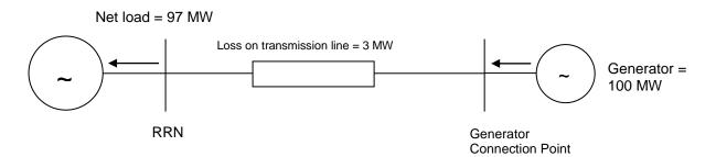
Figure 5: Radial network prior to 1 MW load injection at generation connection point
