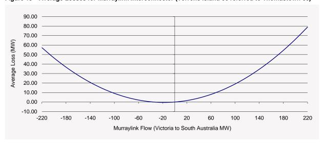
Murraylink notional link losses versus Murraylink flow (Victoria to South Australia)
