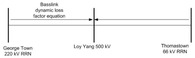
The equation describing the losses between the George Town 220 kV and Loy Yang 500 kV connection points can be determined by integrating the (loss factor equation – 1), giving:
