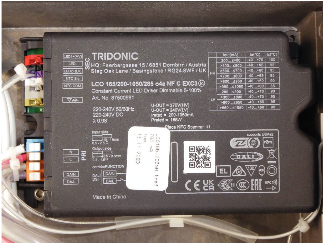
LED driver (Tridonic, LCO 165/200-1050/285 o4a NF C EXC3) (model 102-0911)
