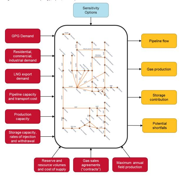
Figure 7 Gas model topology, inputs, and outputs
