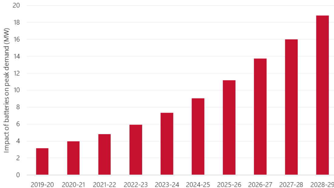
Figure 14 Peak demand reduction from battery storage, 2019-20 to 2028-29 A
