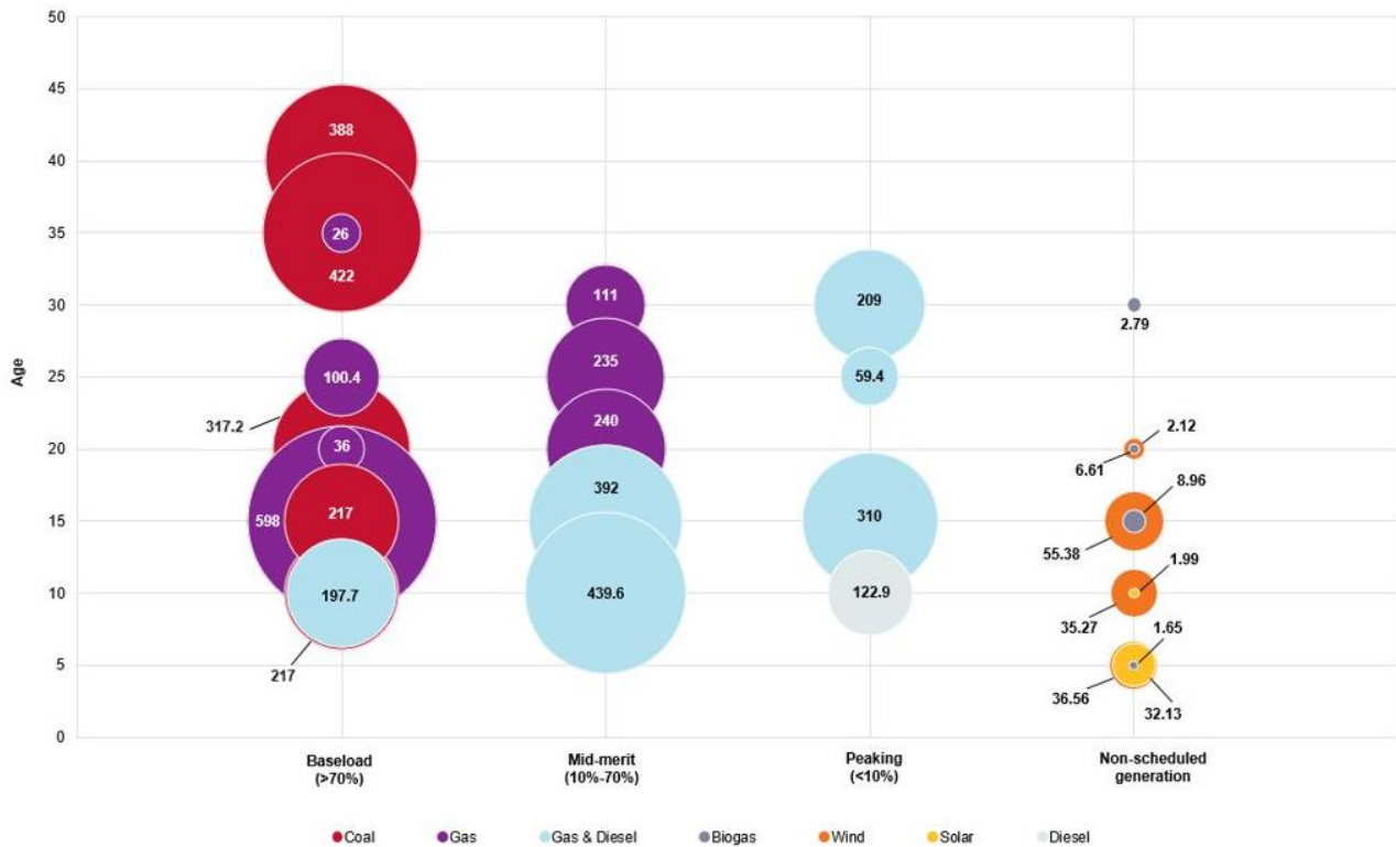
Figure 6 Facilities operating in the SWIS by age, fuel capability, and capacity classification A,B
