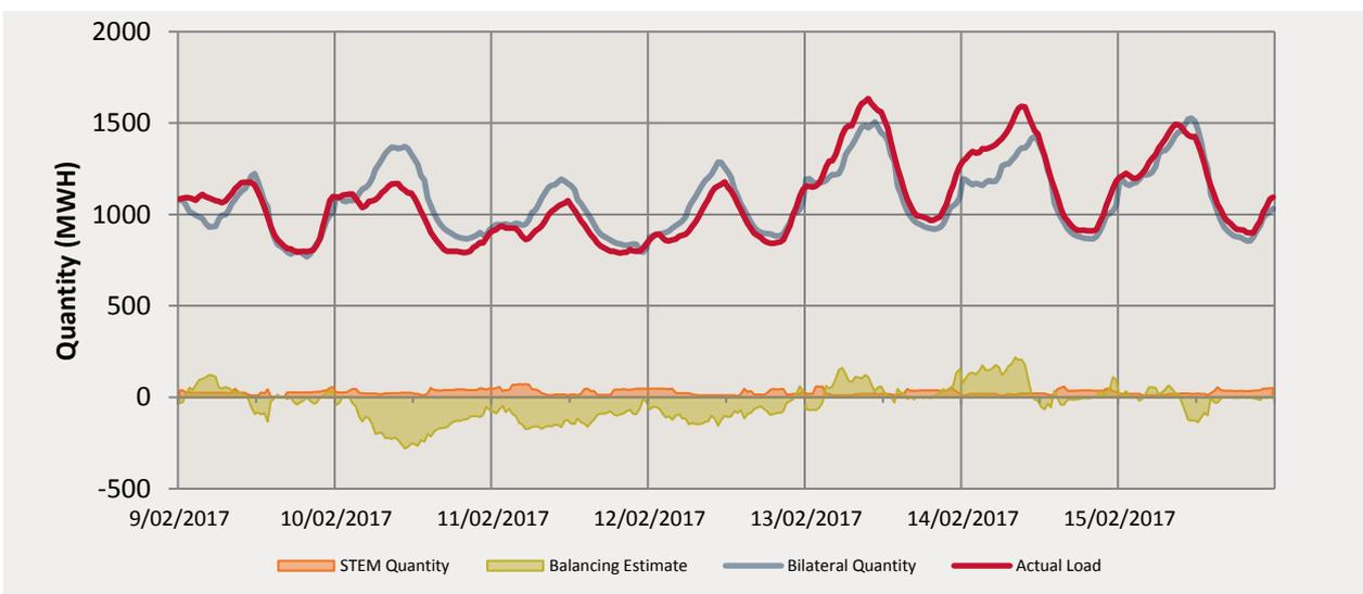
Total balancing supply equalled -19585.572 MWh whereas total balancing demand equalled 7838.986 MWh. The Total STEM Traded quantity was 9459.209 MWh, with the STEM Clearing Quantity ranging between 1.5 MWh and 72.152 MWh.
