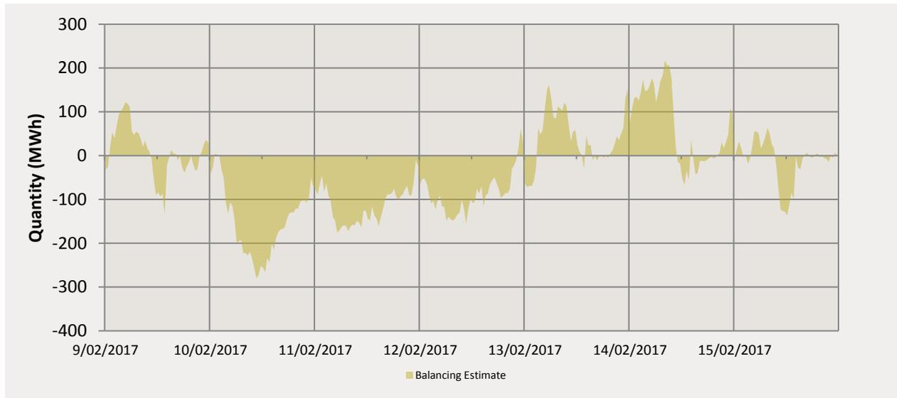
The majority of the balancing activity this week occurred within Balancing Supply. The maximum balancing demand for the week reached 217.51 MWh on the 14/2/2017. The maximum balancing supply for the week reached -280.082 MWh on the 10/2/2017.
