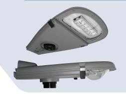
The GE Evolve P4P5 Gen 3 was designed for Australia's P4 and P5 street lighting category and complies with SA/SNZ TS 1158.6:2015. GE's latest LED roadway fixture builds upon the successful Evolve P4P5 and by using the latest LED and driver technology delivers both improved efficiency of 135 lumen per watt and increased driver life to 100,000 hours. Plus, we now offer the option of 1-10V and DALI dimming. Supplied with 7-pin NEMA socket to provide future compatibility with Smart Networking.
