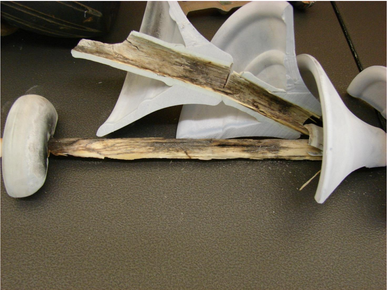
Figure 3 Damage caused by flashover occurring underneath the rubber sheaths
